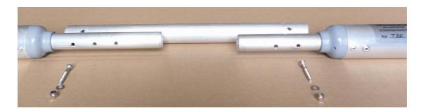
Longer antenna lower the resonance, shorter antenna increase the resonance. In both cases will have effect on the others lower bands. Start the eventual calibration always starting from the highest frequency (10m - 15m - 20m - 40-).
