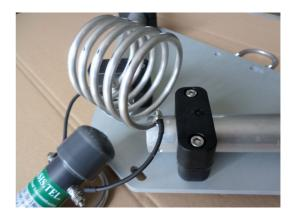
Connect a 1:1 balun to the dipole center (recommended) with two wire jumpers no longer than 8-10 cm (the length affects the resonance of all bands), if you decide not to use the balun, connect terminals of the coaxial opening it as a V directly to the two bolts. Even in this case to make sure that the two terminals of the coax does not exceed 10cm. If too long, the antenna will resonate slightly lower. Seal the coax with good quality sealing glues.
